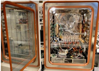
Test of PEM fuel cells in a climate chamber
