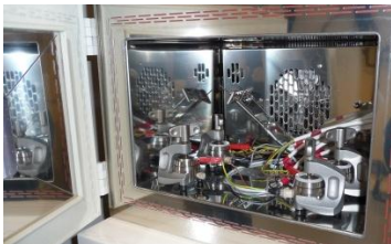
Test cells with reference electrode in climate chamber
