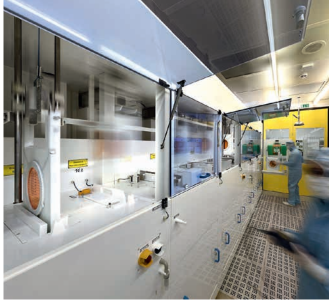
Semi-automatic electroplating tool with five different plating baths (100–300mm wafer size)
