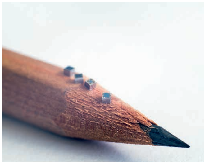
Piezoresistive pressure sensor with 0.8 mm 2 footprint
