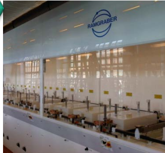
Automatic plating line
