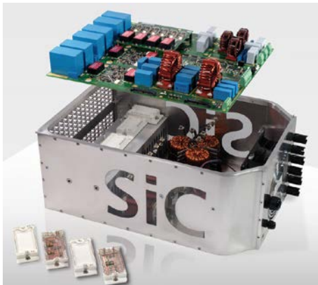
IZM Gen.1 (2012) SiC JFets, 48 kHz pulse frequency 18l - 18,4 kg (15kW) Conventional Packaging
