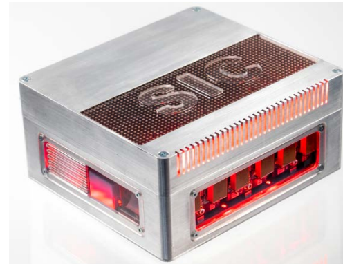
IZM Gen.2 (2015) SiC MOSFets, 250 kHz pulse frequency 2,4l - 4 kg (15kW) Embedded Power modules
